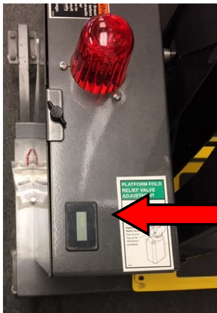
Motor Housing on the side of the lift
